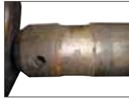
Severe wear to pin
