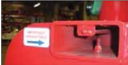
New position of grease point on end of saddle
