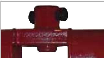
Severe wear to pin
