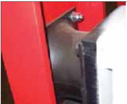
New position of grease point on end of saddle
