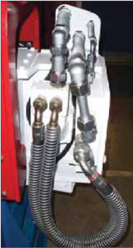
Severe damage to hose assembly
