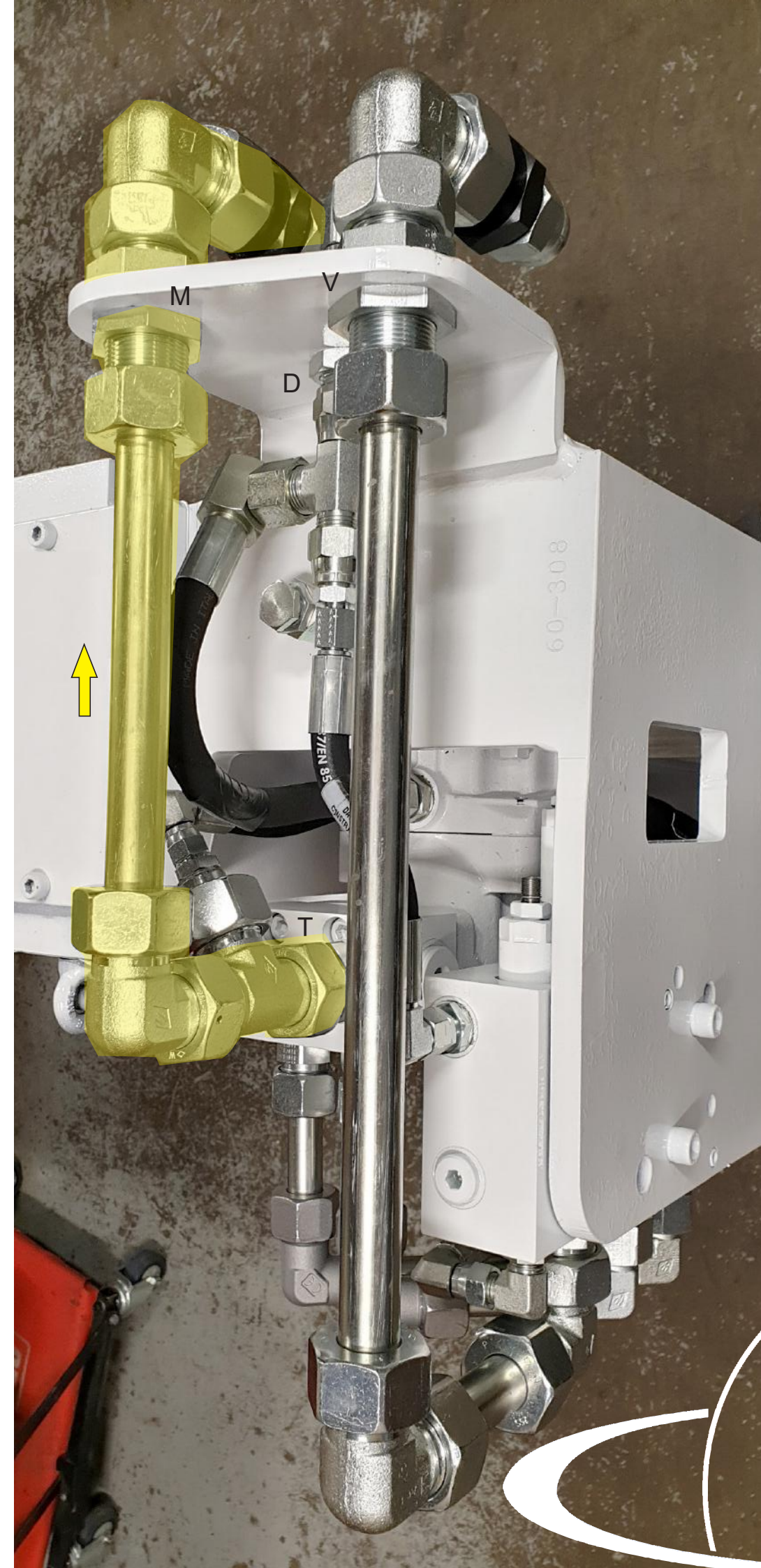
emv450 JIC hydraulic circuit
